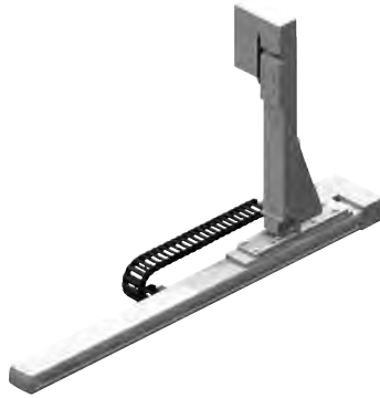
Wiring 1 with cable track
